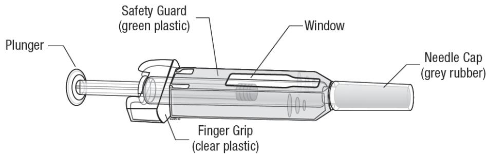
Activate the green safety guard (slide over the needle) after the injection.
